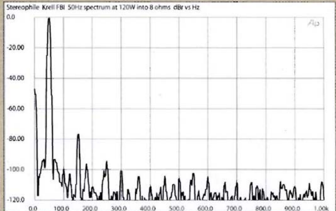
Fig.6 Krell FBI, spectrum of 50Hz sine wave, DC-1kHz, at 120W into 8 ohms (linear frequency scale).
